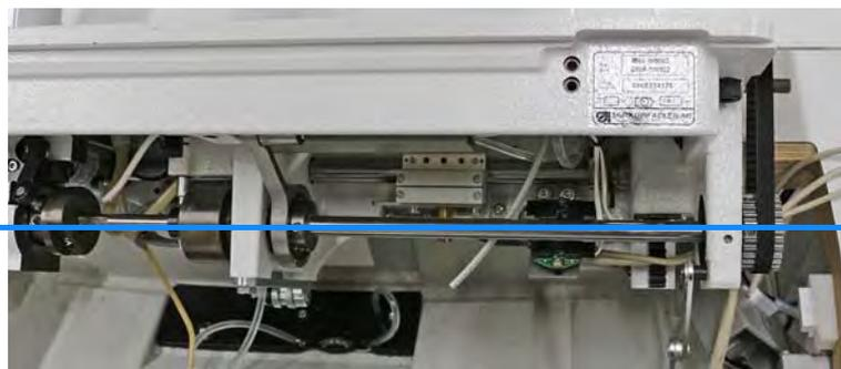
The toothed belt is positioned correctly when the screw in the lower toothed belt wheel lines up with the screw in the eccentric and in the set collar AND when it is positioned next to the marking in the machine casting.
