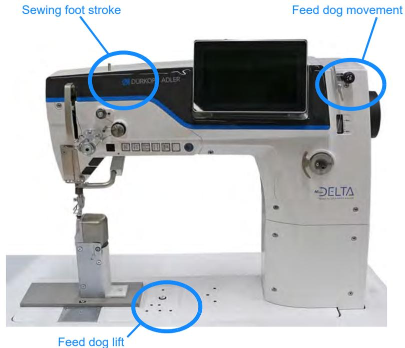
The *looping stroke* securing position allows you to define the basic settings for the **sewing foot stroke**, the **feed dog lift** and the **feed dog movement**.
