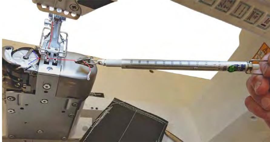
The holding force of the hook thread clamp is measured by looping the needle thread around the hook thread and pulling it through the needle hole. Next, the force is measured with the help of a spring balance.
