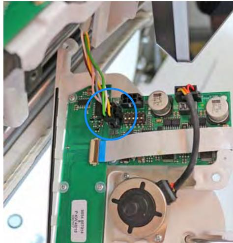
On 2-needle machines the plug of connection **X103** must be detached from the PCB found behind the thread tension plate.
