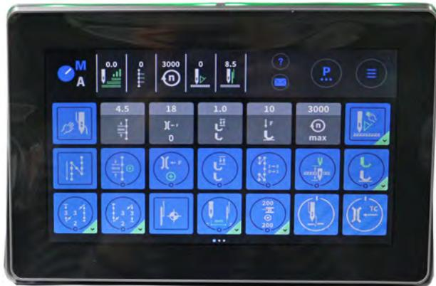
All settings in the software are performed using the Commander DELTA control panel.
