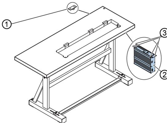
(1) - Strain relief mechanism
