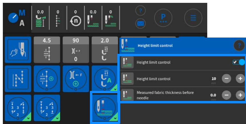
Fig. 13: Checking the height limit
