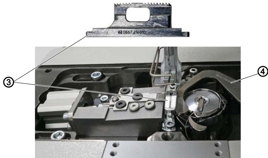
Fig. 8: Assembling the NSB into the machine (3)
