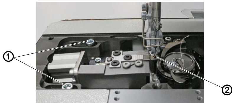
Fig. 7: Assembling the NSB into the machine (2)
