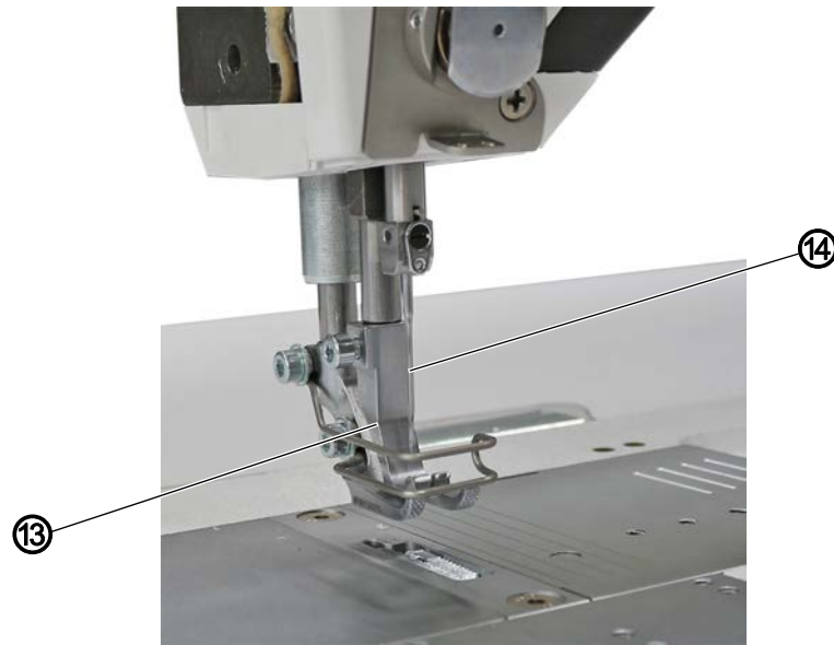
Fig. 4: Assembling the needle cooling (4)
