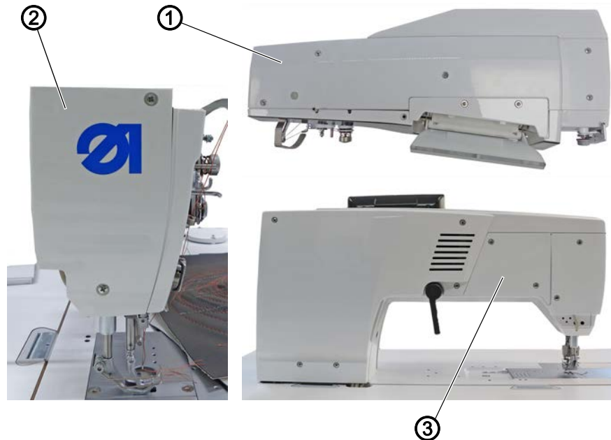
Fig. 6: Assembling the two-axis electronic edge guide (1)
