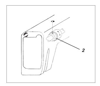
The pressure foot should reach lower dead center together with the needle bar. The upward movement of the pressure foot begins only after the looping stroke.
