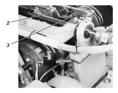
During the folding sequence the fixed clamp presses the interior slide first against the hold-down and then against the swung-in outer forward slide 1 at half pressure.
