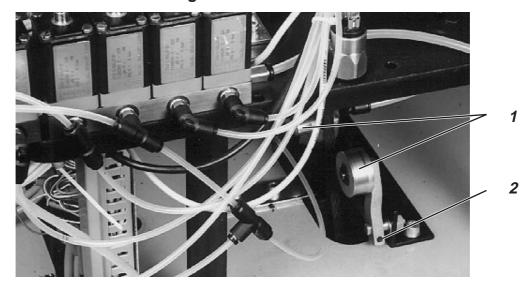
The two contact rollers 1 prevent the timing belt from jumping off the belt pulley when the sewing head is raised.
