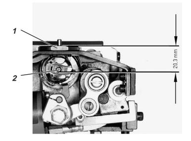
In the **upper position** there is a clearance of 27.7 mm between the upper edge the needle plate 1 and the lower edge of the pin 2.
