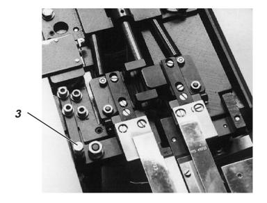
During folding the fixed clamp 1 (clamping table left) is pressed against the hold-down and then against the outer forward slide with half pressure.
