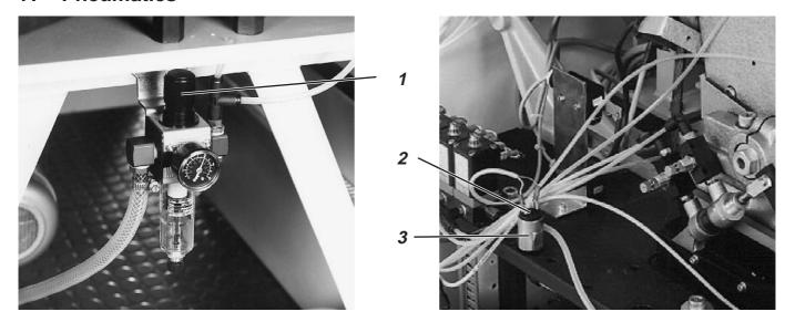
The operating pressure for the pneumatic system of the sewing unit is set at 6 bar by the maintenance unit.
