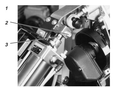
With lowered sewing arm 1 the clearance between the milled bottom of the sewing arm and the lower arm surface should be 72.5 mm.
