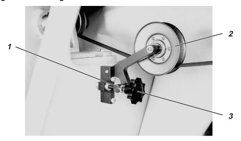
The tension pulley 2 on the V-belt determines the stitch length.
