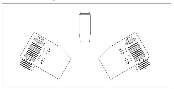
The switching disks no.s 1 to 10 trigger the function of various clamping table elements via the pneumatic valves.
