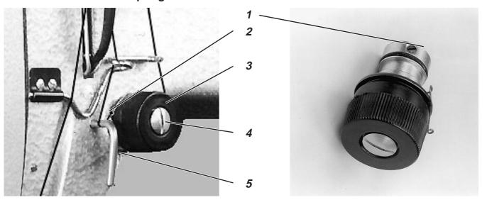
The thread controller spring 2 should have just reached its lowest position when the needle has entered the cloth up to the eye.
