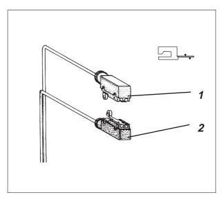
In the upper position of the needle plate switch 2 ( b20 ) should be triggered by the strip 3.
