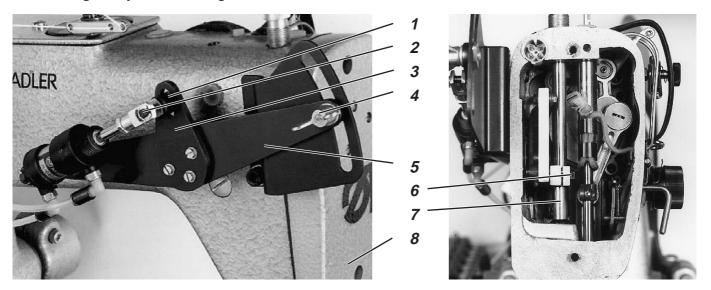
When the lowest stroke position is in effect the pressure foot at the lower dead center should have a clearance of 2.5 mm to the needle hole mushroom.
