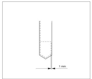
The position of the clamping table determines the position of the seam formation on the trim.
