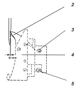
In the looping stroke position the hook point 2 lies at the center of the furrow.
