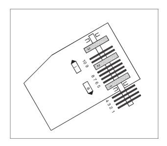
The switching disks no.s 1 to 10 are arranged as per the setting disk. The switching disks no.s 3 to 10 are deployed as pairs (3 + 4, 5 + 6, 7 + 8, 9 + 10).
