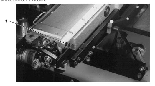
The knife should securely cut with the least possible amount of pressure.
