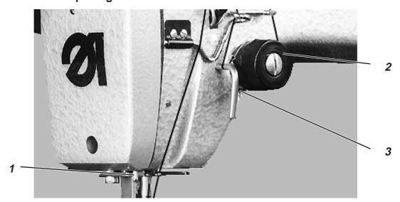
The thread tension opening occurs during the trimming sequence via the magnet in the head cover or manually by pressing the pin 1.
