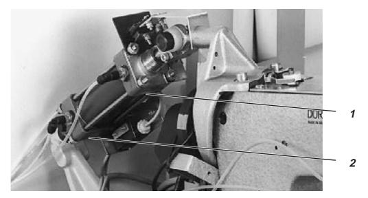
The speed of the piston rod is reduced approx. 10 mm in front of the end position in order to softly brake the heavy sewing head.
