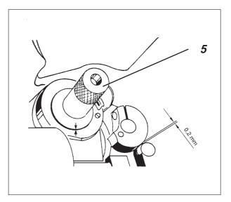
The height of the base plate determines the clearance of the thread pull knife to the hook.
