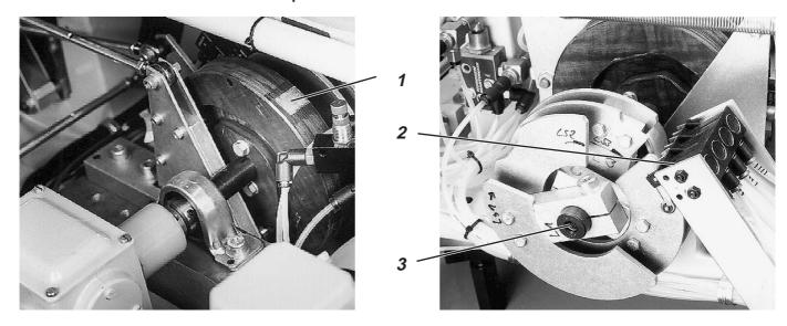
The aluminium strips 1 on the faces of the 3 guide curves stop their turning movement according to the function sequence.
