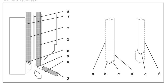
The interior slides 1 and 2 determine the clearance between the seam and trim edge in the following seam segments.
