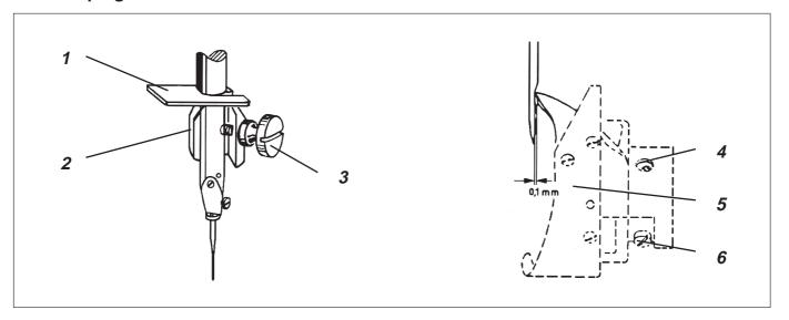
The looping stroke is the path of the needle bar from lower dead center up to the point where the hook point lies at the center of the needle.
