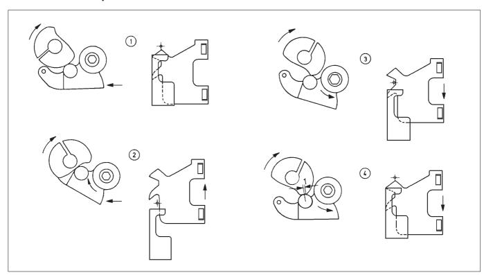
When, after the "seam end" signal, the 1st position is reached, the thread trimmer magnet is switched on and the drive segment pressed against the guide curve. The thread tension is opened and the sewing unit runs at the cutting rpm of 160 min<sup>-1</sup>.
