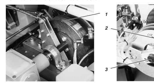
The guide curve no. 1 should, after a turn of 20°, start with the forward movement of the side slides of the fixed table.
