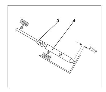
In the upper position of the sewing arm switch 2 (b17) should be triggered.
