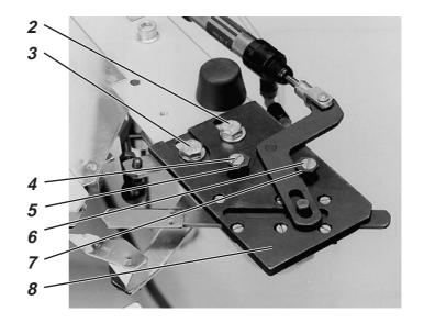
The inner forward slide 1 folds the trim around the interior slide. Then the center forward slide folds the trim around the inner forward slide.
