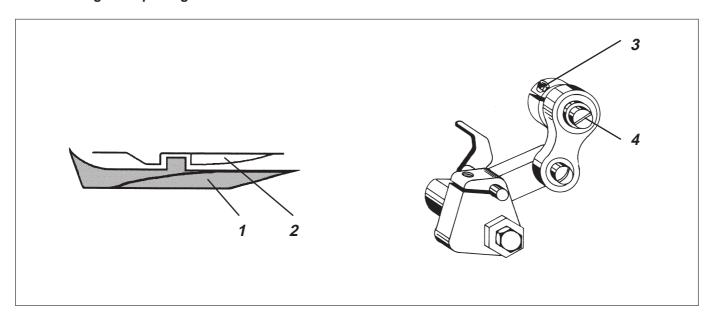
The middle piece should be opened at the moment the thread slips through between the middle piece 2 and its holder 1.
