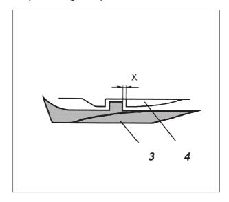
The gap x between the opened middle piece 4 and its holder 3 should be appropriate for the thickness the thread to be sewn.
