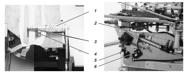
The hold-down 1 is manually swung upward and presses the interior slides down against the clamps.
