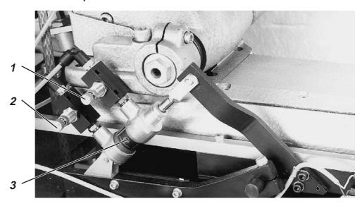
The needle plate is brought into the upper or lower position by cylinder 3.
