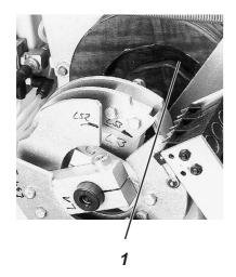
The 3 guide curves no.s 1 to 3 mechanically trigger the functions listed in the table via the inner and outer curve runs 1.
