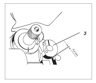
When the drive segment 4 is swung completely back there should be a clearance of 0.2 mm between it and the guide curve 3.
