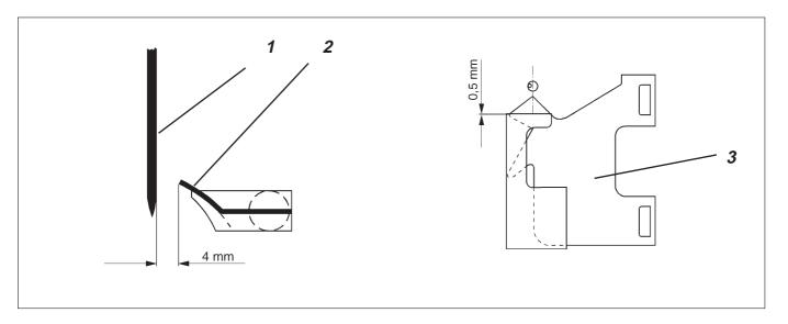
The clearance of the counter knife 2 to the needle 1 should be 4 mm. The position of the thread pull knife 3 to the counter knife determines the knife overlapping and the timing of the cutting.
