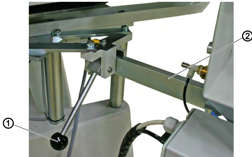
Fig. 34: Connecting the stacker to the sewing unit
