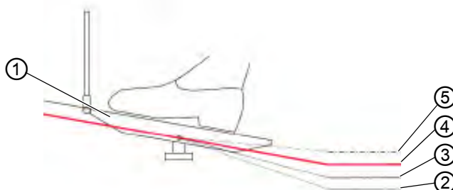
Fig. 25: Lifting the sewing feet electropneumatically
