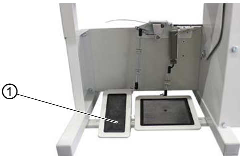
Fig. 20: Lifting the sewing feet with the pedal
