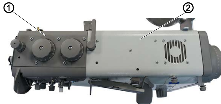
Fig. 4: Disassembling the old tensioning plate
