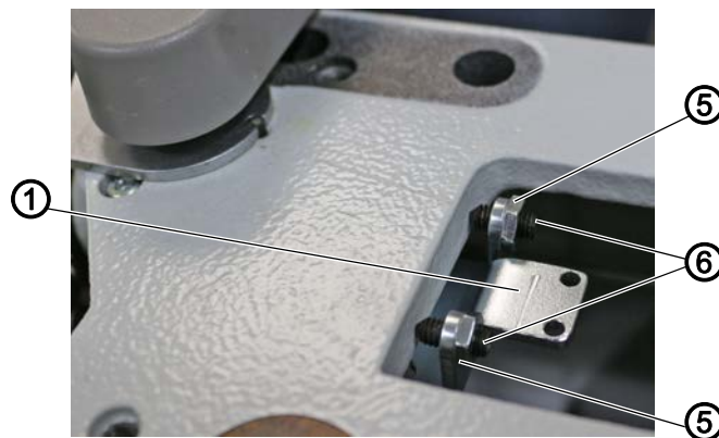
Fig. 10: Assembling the new tensioning plate
