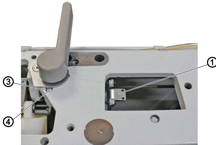
Fig. 9: Assembling the new tensioning plate
