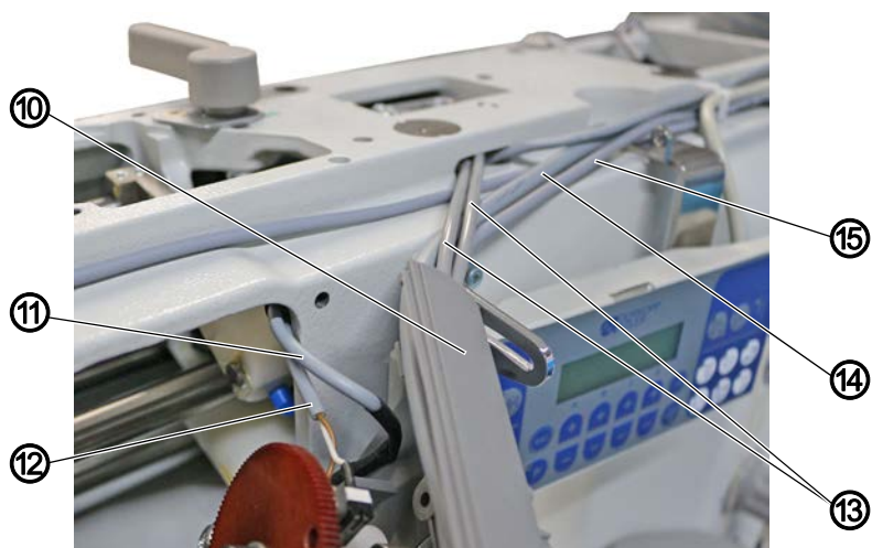
Fig. 13: Assembling the new tensioning plate
