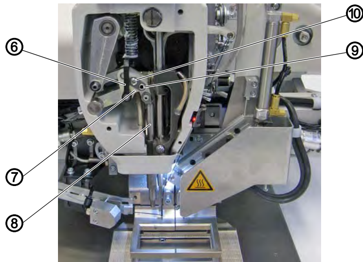
Fig. 66: Changing the cloth pressure bar (2)
