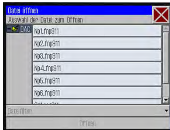
Fig. 88: Opening a seam program or sequence for sewing
