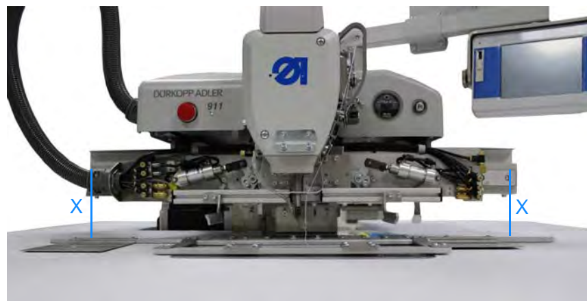
Fig. 12: Aligning machine head (2)
