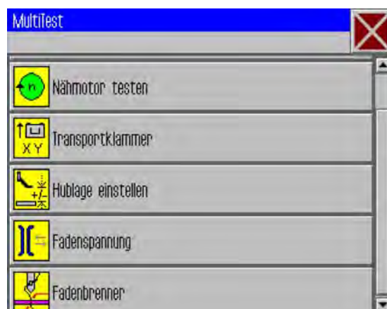
Fig. 106: Testing the functions of the machine
