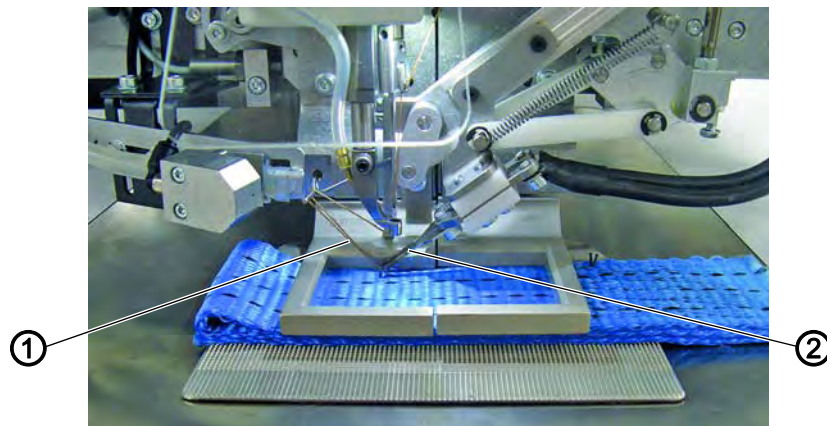
Fig. 50: Setting the upper thread burner
