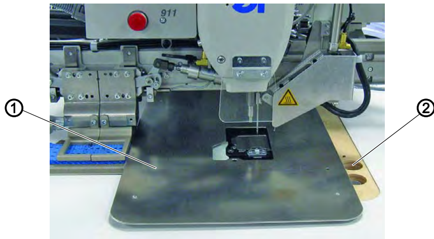
Fig. 8: Removing and placing the sliding plate
