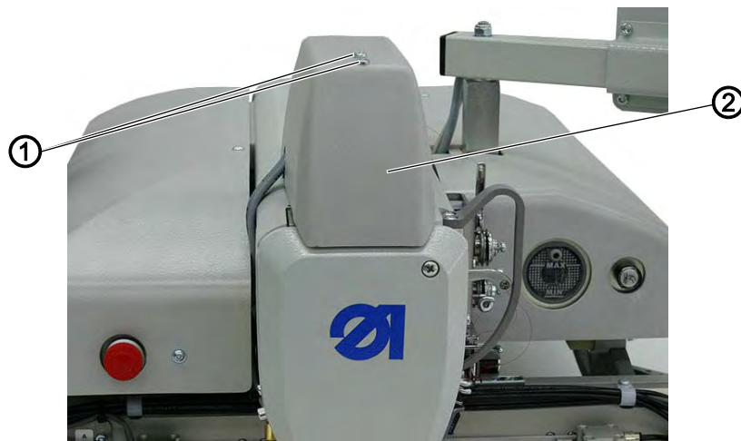
Fig. 2: Removing and assembling the motor cover
