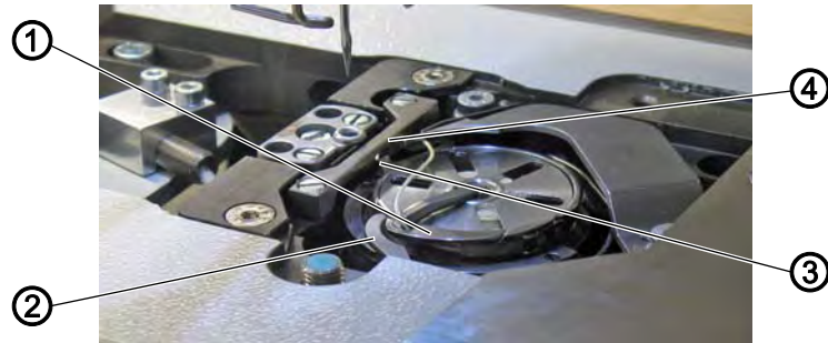
Fig. 30: Setting the bobbin case lifter
