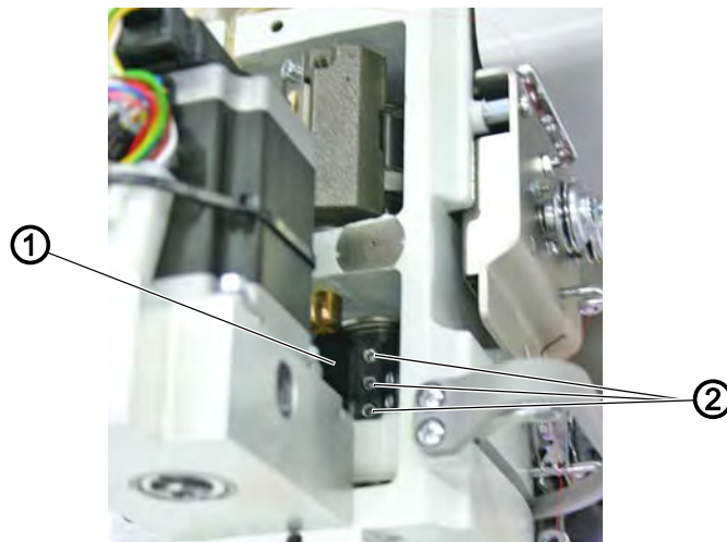
Fig. 20: Positioning the arm shaft crank
