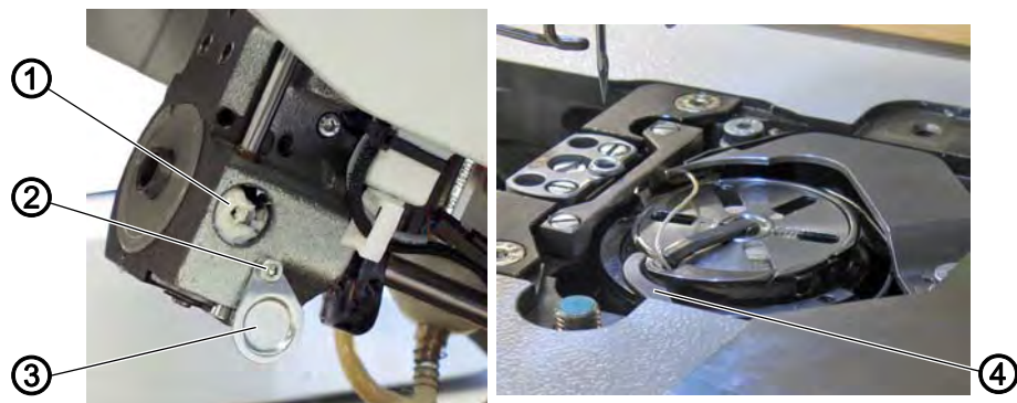
Fig. 31: Setting the lifting gap (standard hook bearing)
