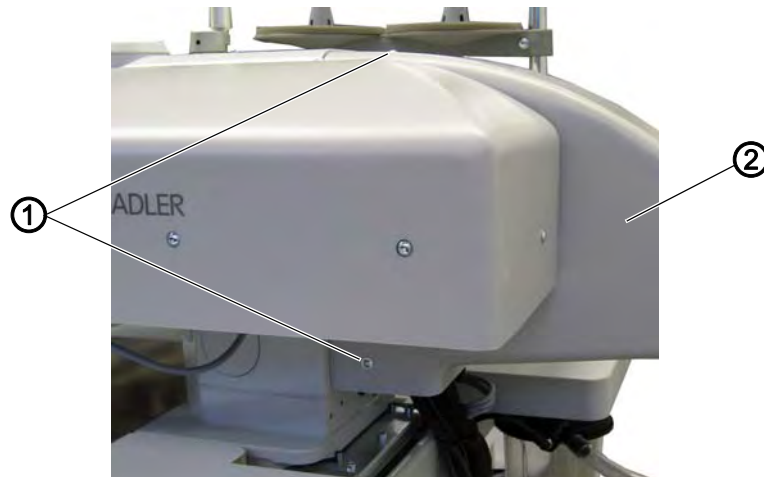
Fig. 5: Removing and placing the rear cover
