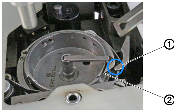
Fig. 31: Adjusting the lifting gap (special hook bearing for safety belts) (1)
