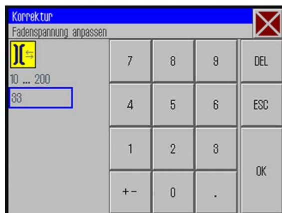
Fig. 32: Sewing with a modified thread tension
