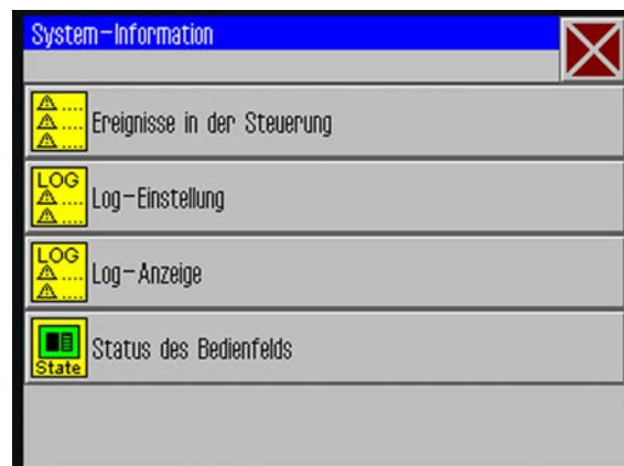
Fig. 55: Calling up log displays and error lists
