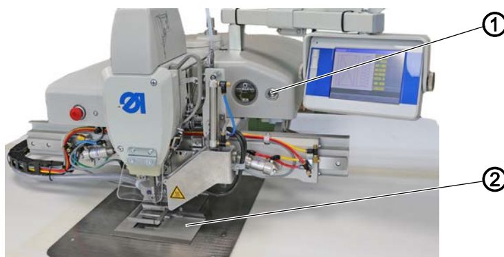
Fig. 5: Switching on threading mode
