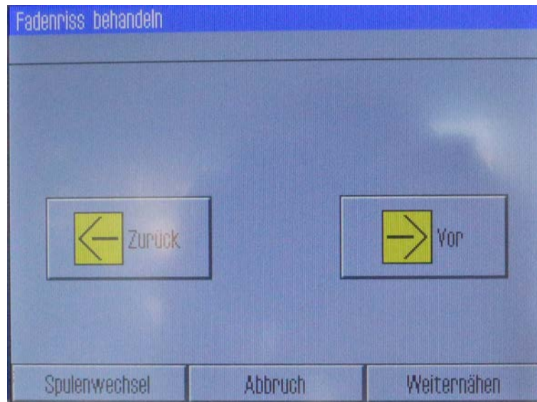
Fig. 36: Continuing a seam after thread breaking
