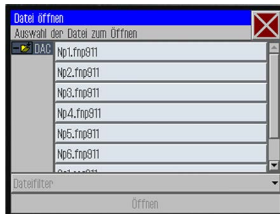
Fig. 31: Opening a seam program or seam sequence for sewing
