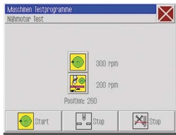
Fig. 54: Testing the sewing motor
