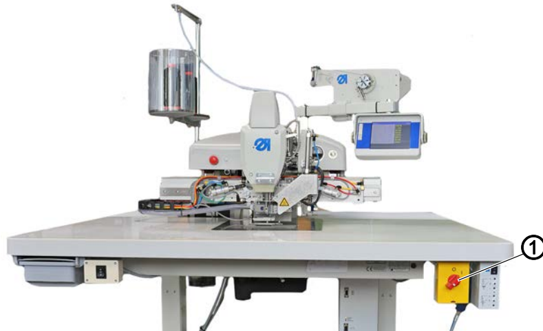
Fig. 2: Switching on and off the machine
