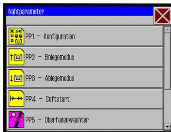
Fig. 43: Changing seam program parameters
