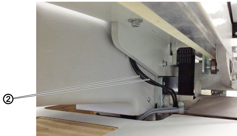
Fig. 2: Assembling the magnet valve (2)
