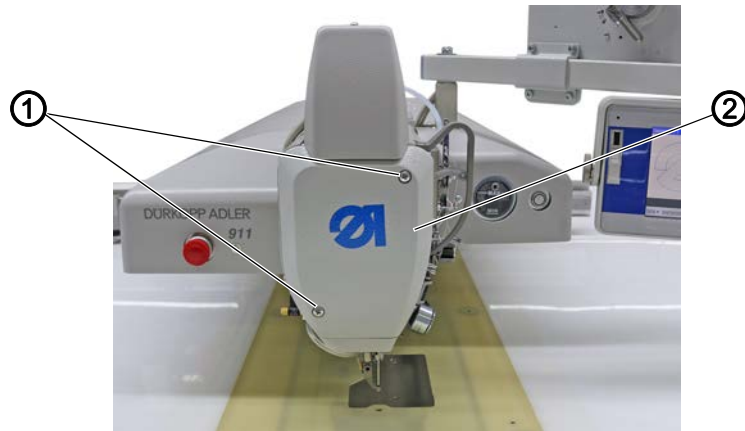
Fig. 3: Disassembling and assembling the head cover
