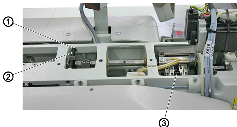
Fig. 32: Adjusting the sewing foot height
