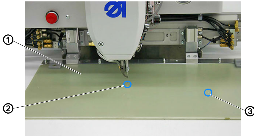
Fig. 62: Checking the machine zero point
