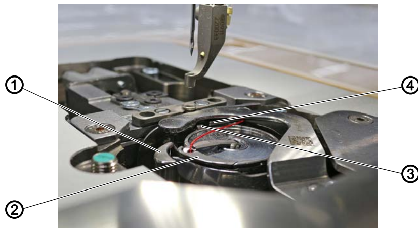
Fig. 25: Adjusting the bobbin case lifter
