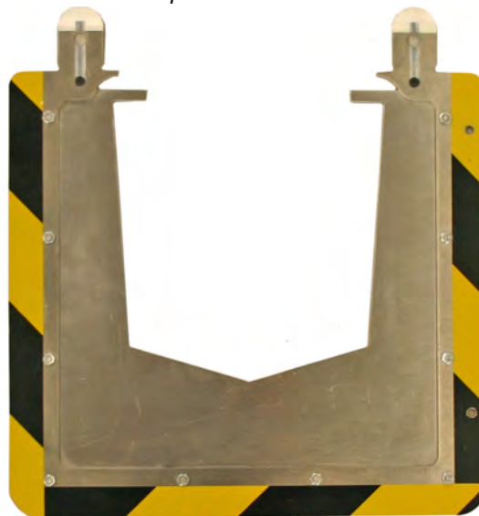
Fig. 15: Cut out outer frame plate
