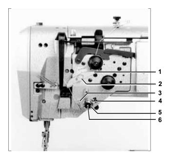
The position of the thread regulator is dependent on the material thickness, thread thickness and the selected stitch length.
