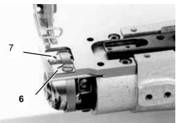
Stepping back on the pedalinitiates the thread trimming process. It runs in 3 phases:
