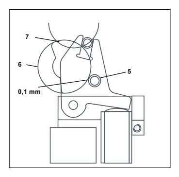
In position **C** (thread lever at upper dead center) the movement of the thread catcher to the counter knife have ended.
