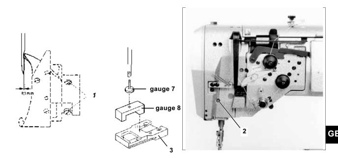
The needle bar height should be so adjusted that the needle point, with a set stitch length of "0" and in the loop stroke position, lies at the middle of the groove.
