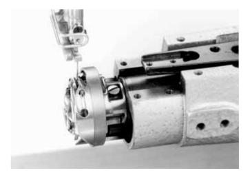
The loop stroke is the distance traveled by the needle bar from lower dead center to the point where the hook tip is at the needle end.
