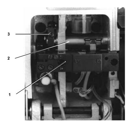
The transporter should make the smallest possible advancing movement when the corresponding adjustment wheel is set at a stitch length of "0".
