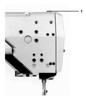
The screw 1 must be screwed in as far as possible so that maximum pressure is achieved.
