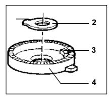
The adjustment wheel can only be turned to the right or left until the stop ring 2 reaches the corresponding cam side of the lock ring 4. When the adjustment wheel is turned completely to the right then:
