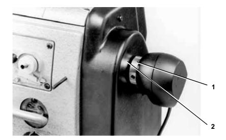
Before setting check if the synchronizer is properly fastened. With the machine arrested in slot **A** (needle bar 2 mm after lower dead center) the locating mark 1 must be opposite notch 2.
