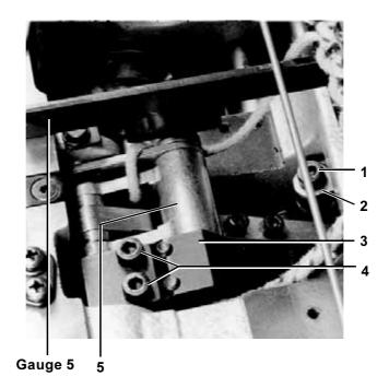
The pressure foot and transport foot lift in the correct relationship at all pressure foot stroke heights which can be set.
