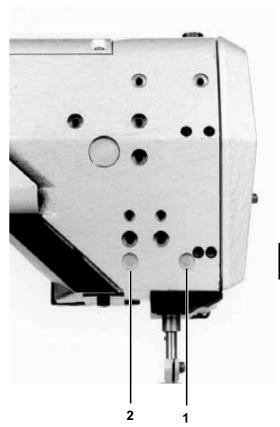
The clearance between the transport foot bar and material pressing bar be 11 mm with the machine arrested in position **E** ( needle bar at lower dead center).
