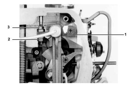
The link holder 1 must be parallel to the lower edge of the arm head.
