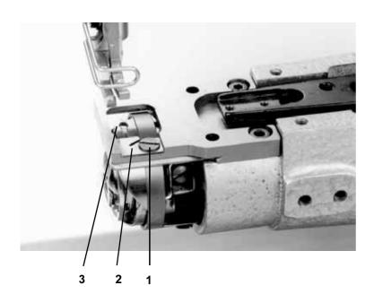
The tip of the thread catcher 2 swung into its initial position should be below the counter knife and have a clearance of 1 mm to the trimming edge of the counter knife.
