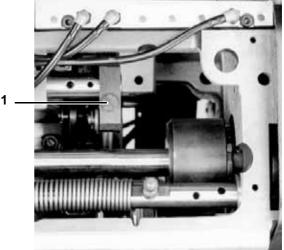
The needle and the transport foot should make the smallest possible advance when the corresponding adjustment wheel is set to a stitch length of " 0 ".
