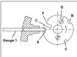
The machine head is equipped with a built-in adjustment disc, which makes possible a quick and accurate adjustment of all elements.
