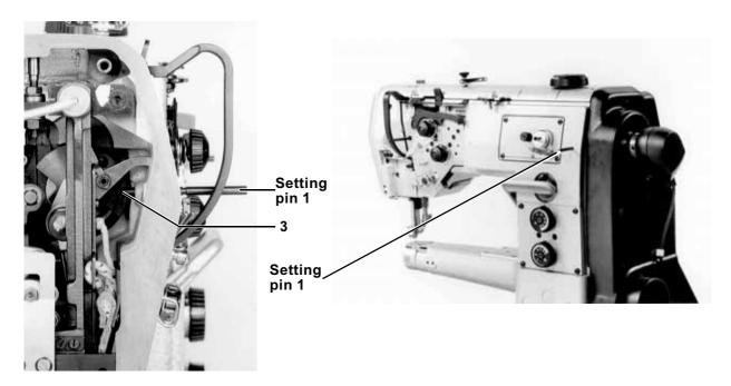
The deepest slot **(A)** of the adjustment disc must be in line with the groove 3 in the arm shaft crank.
