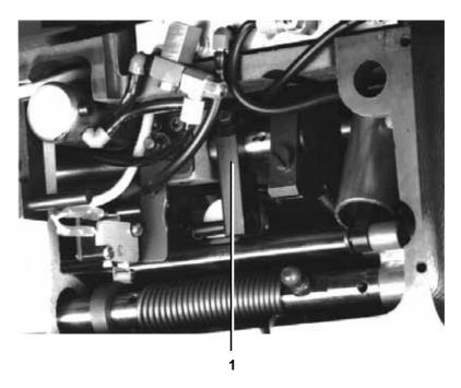
The pressure feet can be raised by stepping back on the pedal.
