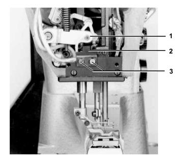
The safety stop 2 is to keep the pressure foot bar and material pressing bar from lowering too far after the removal of both pressure feet and thus blocking the drive mechanism.
