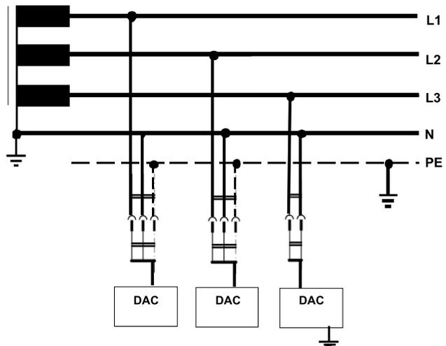
Fig. 6: IT net wiring diagram
