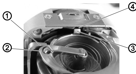
Fig. 29: Setting the opening of the middle part of the hook
