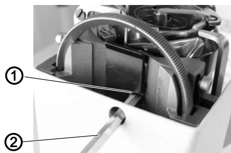
Fig. 27: Setting the needle guard
