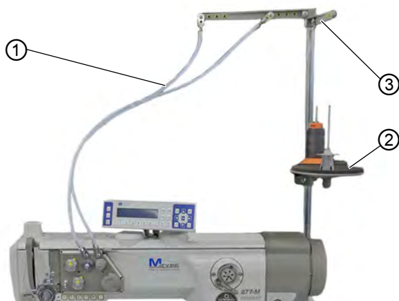
Fig. 8: Winding on the hook thread – part 1
