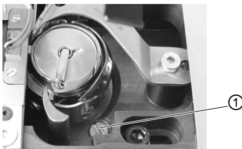
Fig. 72: Lubricating the hook
