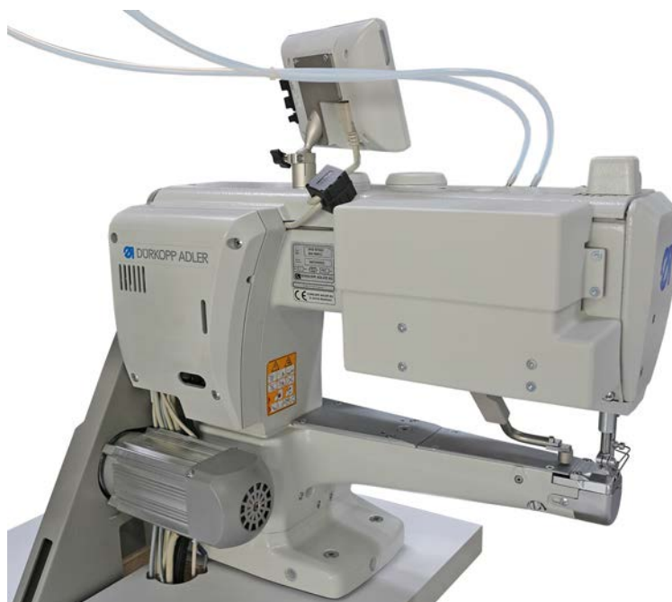
Fig. 12: Assembling the two-axis electronic edge guide (6)
