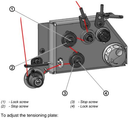
Fig. 2: Adjusting the tensioning plate (1)
