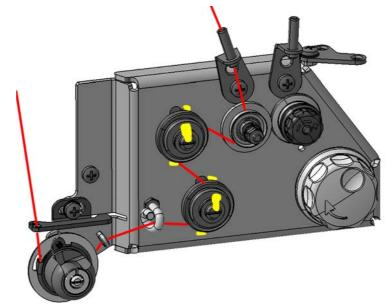
Fig. 7: Checking the adjusted thread tension (1)
