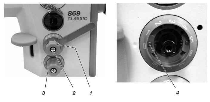
Depending on the sewing equipment used the stitch length setting must be limited to 6 or 9 mm.
