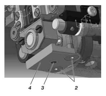
Insert pin 3 on plate 4 (order no. 0869 160123) into the hole on the stroke eccentric and screw in with two screws 2.
