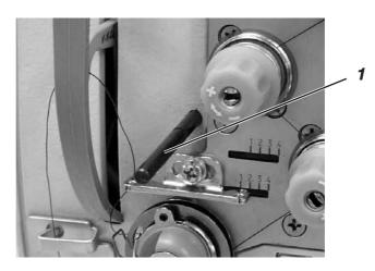
The locking pin 1 required to set the machine is provided as standard with the machine. It is in the machine's accessories' kit and can be fixed to the bottom of the oil sump so that it is easy to get to.
