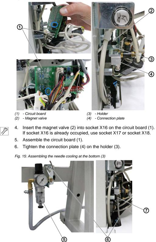
Fig. 14: Assembling the needle cooling at the bottom (2)
