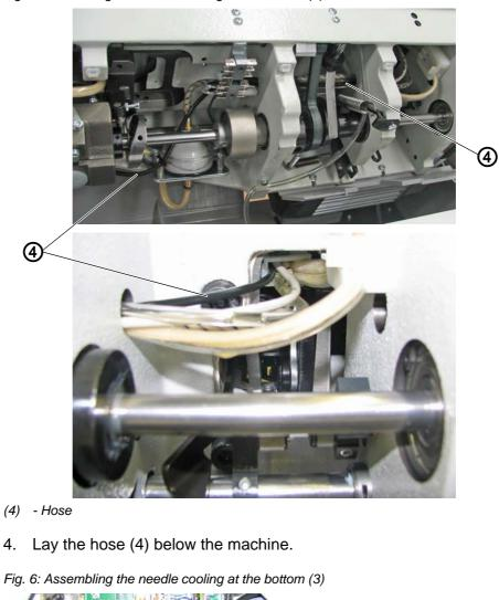
Fig. 5: Assembling the needle cooling at the bottom (2)
