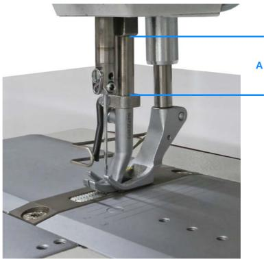
When the presser foot is lowered, the distance **A** must be 26 mm. On machines with short thread cutter the distance **A** must be 24 mm.
