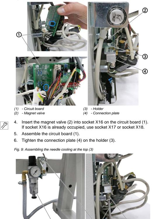
Fig. 8: Assembling the needle cooling at the top (2)
