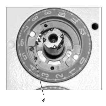
Depending on the sewing equipment used, the stitch length setting has to be limited to  $\bf 6, 9$  or  $\bf 12$  mm.
