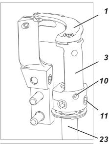
The thread-pulling knife 1 is supposed to swing past the bobbin as close as possible. The distance between the thread-pulling knife and the bobbin should not exceed 0.1 mm.
