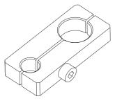
Setting gauge 0868 290194 chapter 2.4 Needle bar linkage chapter 2.5 Post bed feed
