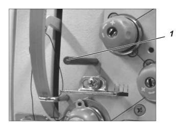
The locking pin 1 required for adjusting the machine belongs to the serial equipment of the machine. It is in the accessories and can be put at the bottom side of the oil pan.
