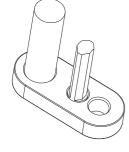
**Setting gauge 0868 290113** chapter 2.4 Needle bar linkage
