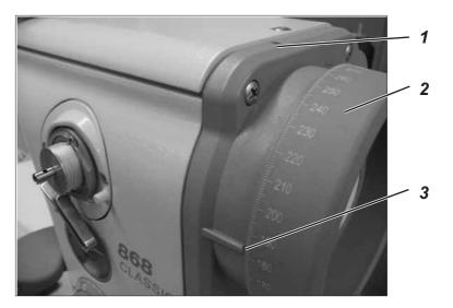
The handwheel 2 has degree marks printed on it.
