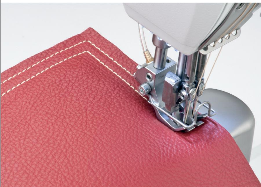
The special M-TYPE subclasses with disconnectable needle bars are ideal operating means for twin-needle decorative stitching applications. Apart from high-quality twin-needle topstitching seams also optically attractive decorative stitch corners can be realized owing to the disconnectable needle bars.
