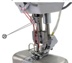
Fig. 15: Threading the needle thread (2-needle machine) (6)
