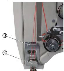
Fig. 14: Threading the needle thread (2-needle machine) (5)
