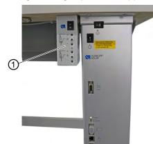
Fig. 101: Connecting the sewing lamp transformer (1)
