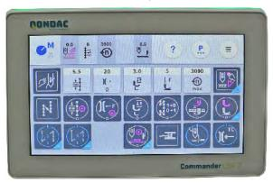
All settings in the software are performed using the Commander Basic/Pro control panel.
