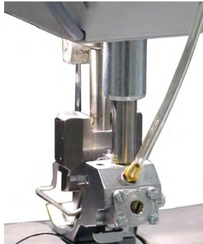
Kit N800 005650 contains an adapter that is used to connect the black pneumatic hose (11).
