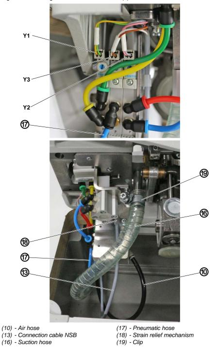
Flg. 13: Assembling the NSB into the machine (8)
