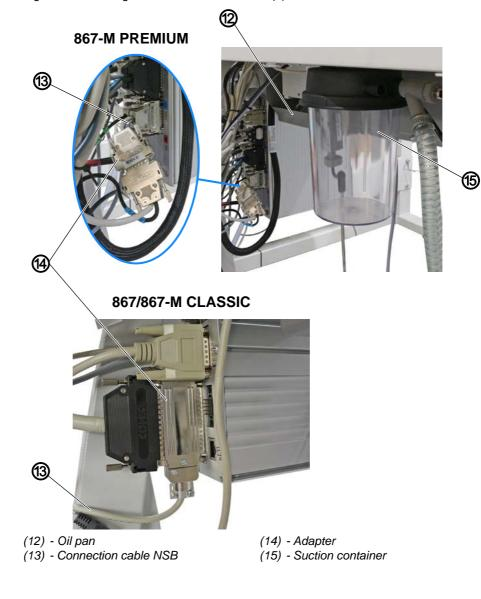
Flg. 11: Assembling the NSB into the machine (6)
