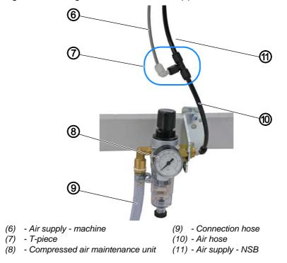
Flg. 10: Assembling the NSB into the machine (5)
