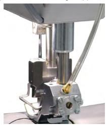
Kit N800 005650 contains an adapter that is used to connect the black pneumatic hose (11).
