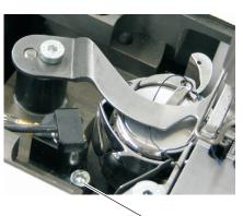
Set the position of the light barrier in a way that its beam goes through the slit of the bobbin case and can be reflected back by the bobbin surface again.
