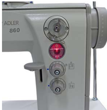
Fig. 59: Checking the oil level (2)
