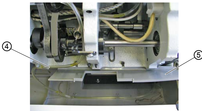
Fig. 84: Assembling the oil extraction line (2)
