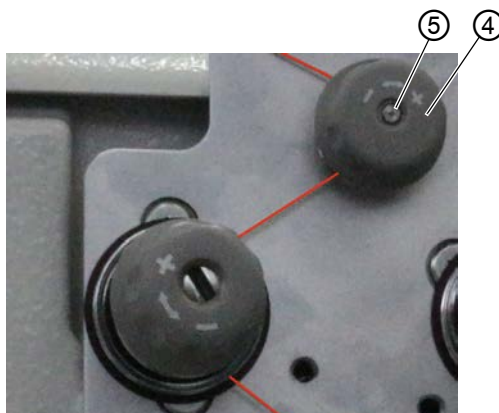
Fig. 29: Adjusting the needle thread tension (2)
