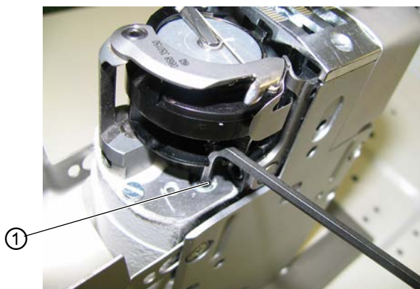
Fig. 60: Adjusting the hook lubrication
