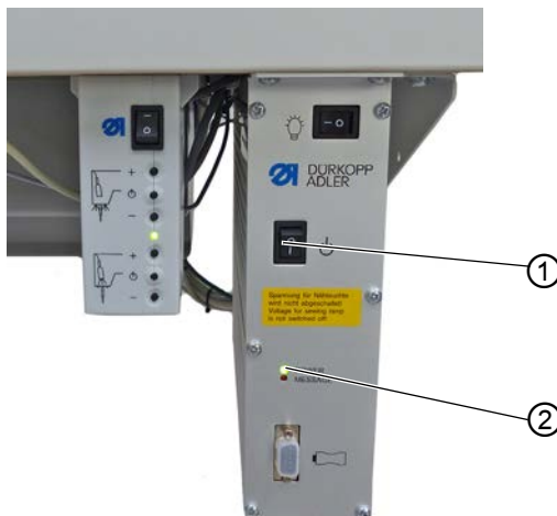
Fig. 2: Switching on and off the machine (1)
