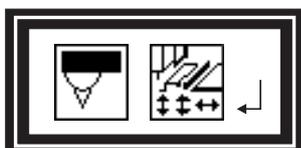
The light barrier 1 checks if material is present. If no material lies under the light barrier, the indicator at the left appears in the display. The indicator can appear under following conditions:
