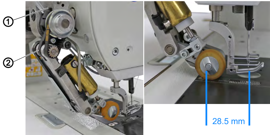
Fig. 49: Adjusting the distance between carrier roller and needle
