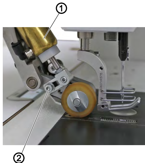
Fig. 51: Adjusting the carrier roller pressure
