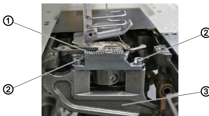
Fig. 23: Moving the feed dog on the feed dog carrier
