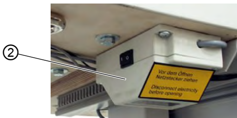
(4) - Sewing lamp transformer
