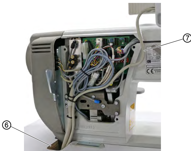
Fig. 35: Assembling the control panel (2)
