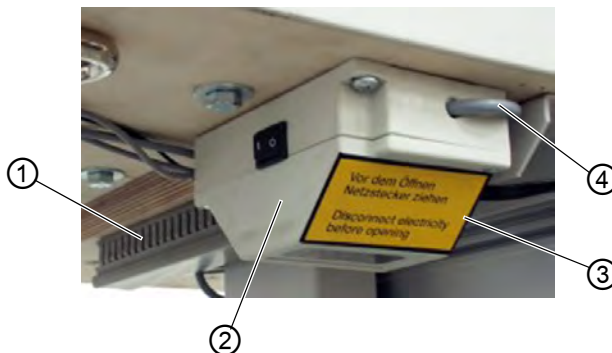
Fig. 42: Assembling and connecting the sewing lamp transformer (1)
