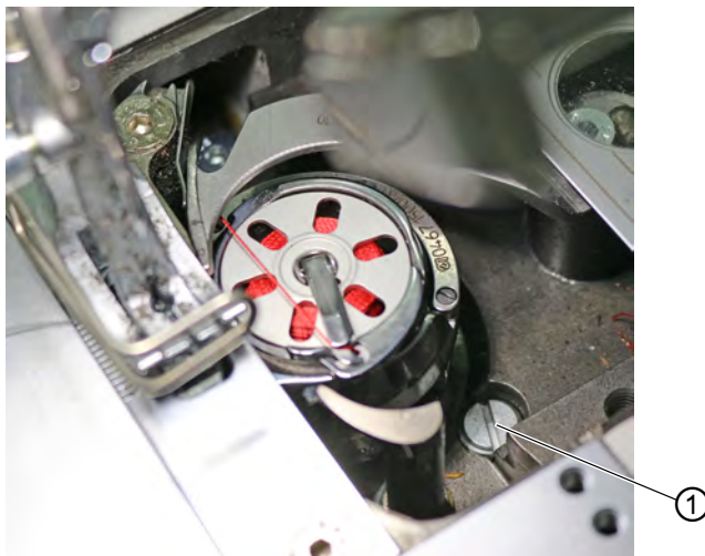
Fig. 25: Lubricating the hook
