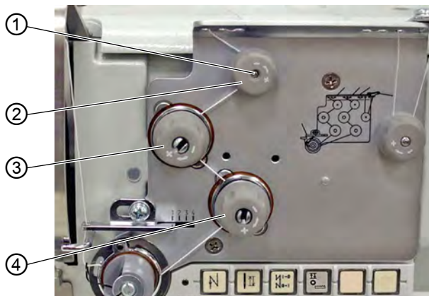
Fig. 10: Setting the needle thread tension
