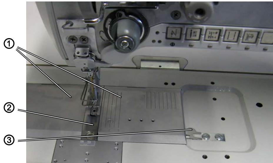
Fig. 5: Opening and closing the throat plate slide
