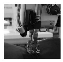
In order to be able to operate the seam center guide the sewing drive DC1600/DA82GA is required.
