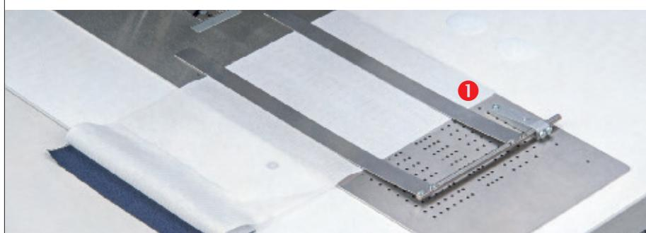
**Suction device** (vacuum 0755 590554) for precise positioning of the workpiece. If there is no central vacuum supply available the vacuum fan (9880 755014) is also required.
