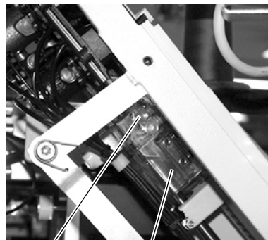
Fig. 56: Oil reservoir hook lubrication
