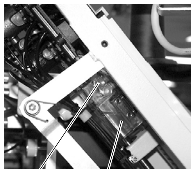
Fig. 72: Oil reservoir for the hook lubrication
