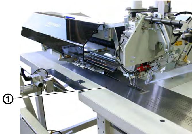
(1) - Edge of the sliding plate (measuring line)
