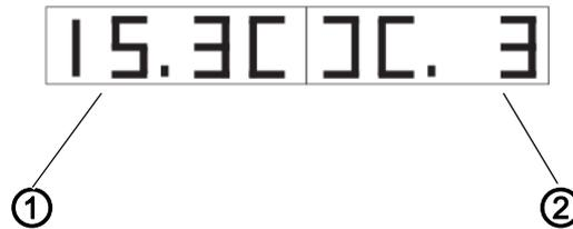
(1) - Value left residual thread monitor      (2) - Value right residual thread monitor
