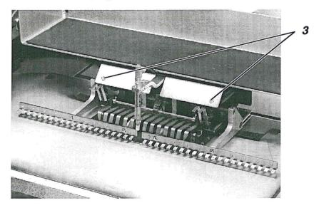
With a normal work sequence one starts with the sewing of the right facing to the collar. The positioning occurs at the left positioning point.
