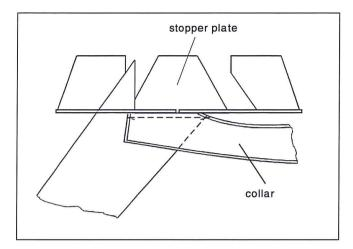
With pointed cut processing the 1st partial seam must be displaced by the width of the seam at the rising cut at the seam beginning and the 2nd partial seam at the seam end.
