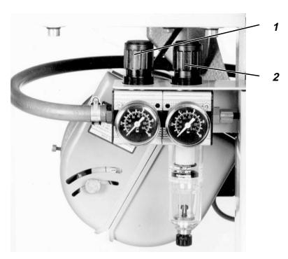
To set the pressure, lift and turn the appropriate knob.
