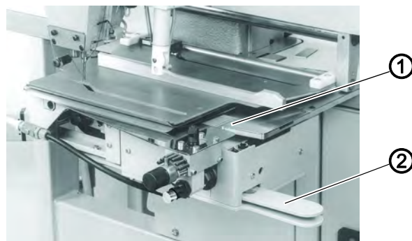
Fig. 15: Setting the working range, angle and length
