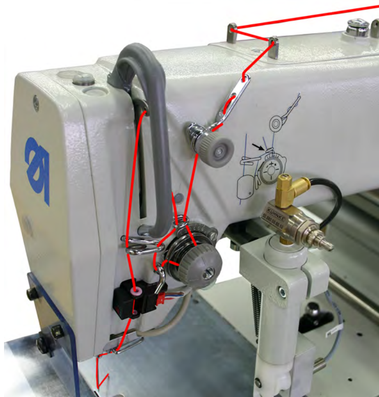
Fig. 5: Threading the needle thread
