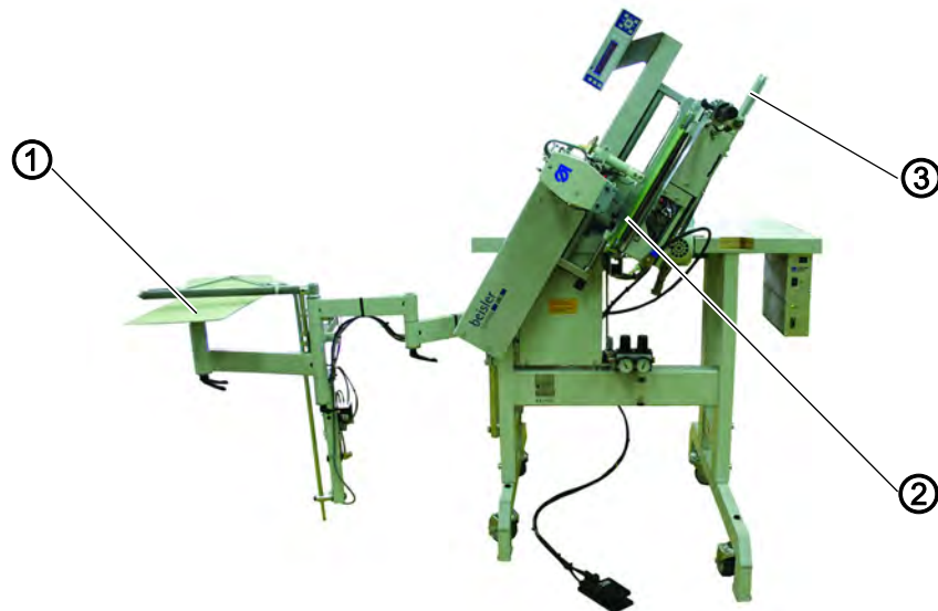
Abb. 23: Swiveling up the machine head
