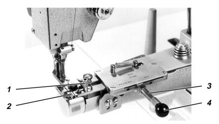
The rapid-adjustment welt-guide mechanism with three positions is used to sew welts between two layers of material. It can be swivelled in or out at the beginning and end of the seam.
