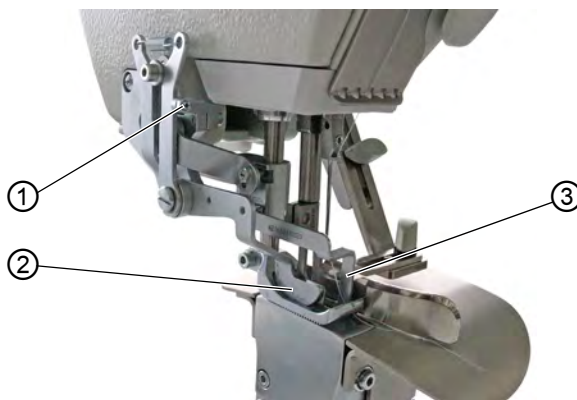
Fig. 24: Setting the height stop for the stitch loosening device
