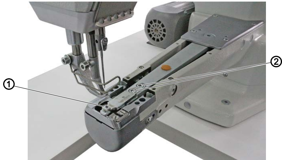
Fig. 10: Disassembling and assembling the feed dog
