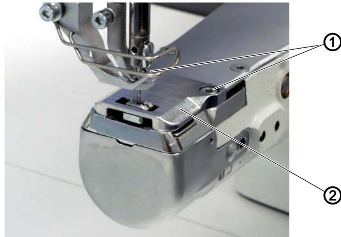
Fig. 9: Disassembling and assembling the throat plate
