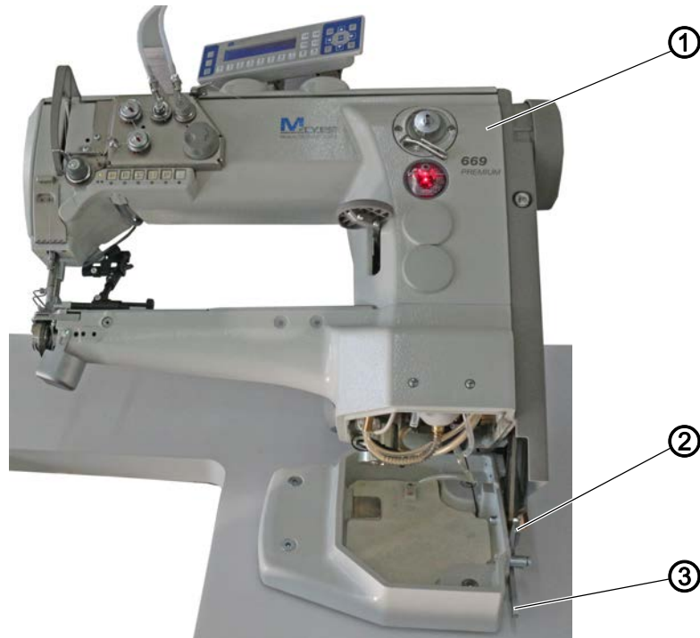
Fig. 5: Tilting the machine head
