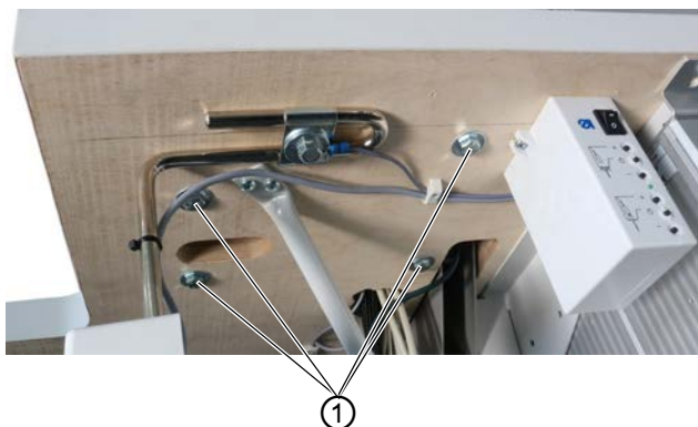
Fig. 57: Placing the machine head (1)
