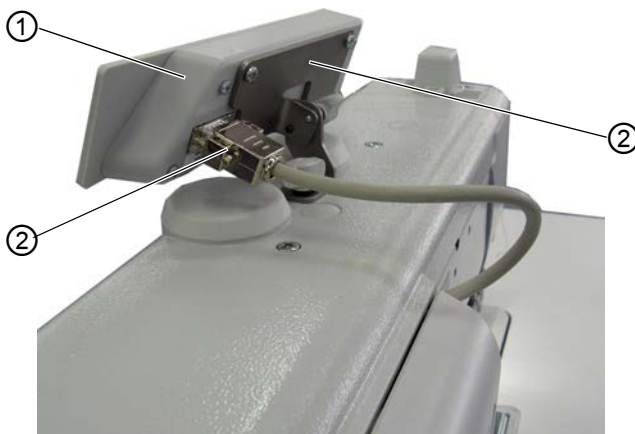
Fig. 58: Assembling the control panel
