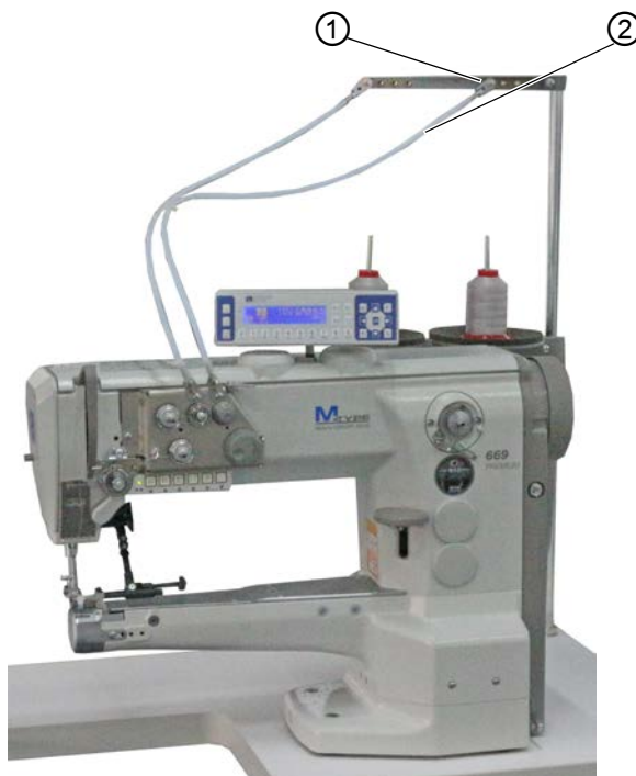
Fig. 9: Winding the hook thread (1)
