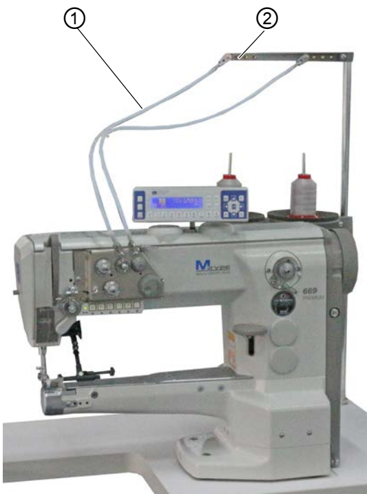
Fig. 5: Threading the needle thread (1)
