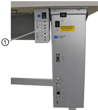
(1) - Sewing lamp transformer
