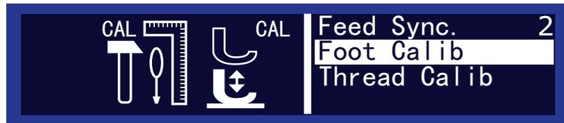
The control unit must know the top and bottom positions of the sewing feet. The top position is sent on switching on the machine.
